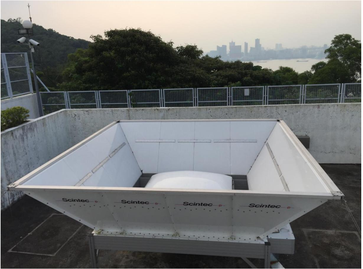
Figure 2 Wind Profiler radar
